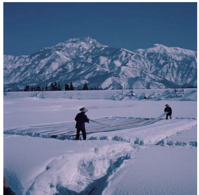
Ojiya-chijimi, Echigo-jofu: techniques of making ramie fabric in the Unuma region of Niigata Prefecture include exposure of the wet fabric to snow
