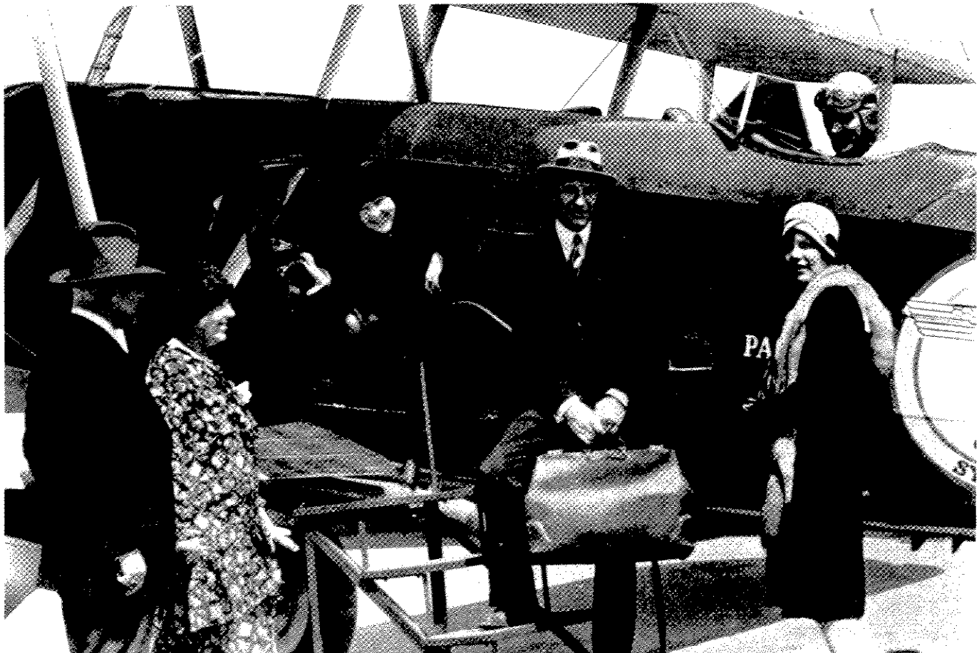
Below: Boeing 40B-4, flown by Pacific Air Transport (PAT) over the coastal and valley routes between Seattle and Los Angeles, carried four passenger seats in a forward cabin area between the wings. The pilot flew in an open cockpit and soared along at 110 miles per hour. The 40B-4 entered service in late 1936 and eventually gave way to the tri-engine Boeing 80 in the early thirties. (Photo from United Airlines Archives)
