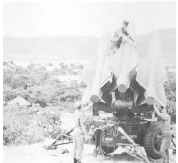
Marine Corps Photo A421300 Marines of the 2d Light Antiaircraft Missile Battalion at Chu Lai make adjustments to three HAWK missiles mounted on their pod. These mobile, surface-to-air guided missiles were designed to defend against enemy aircraft flying at low altitudes.
