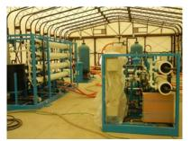
Water desalinations (RO membrane module)
