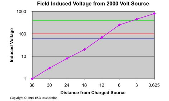
Figure 5 - Voltage Induced onto a 20 pF parallel plate capacitor from a 2000 Volt Uniform Voltage Source at Varying Distances
