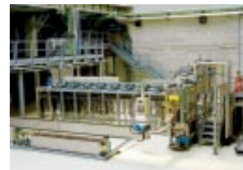
A phase in the CCM (Continuous Compound Mixing) process for the automated production of tyre compounds.
