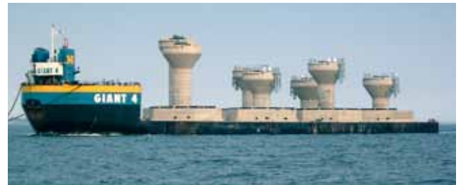
SMIT Transport's "Giant 4" loaded with the concrete wind turbine foundations for the Sprogø windfarm, west off Copenhagen.
