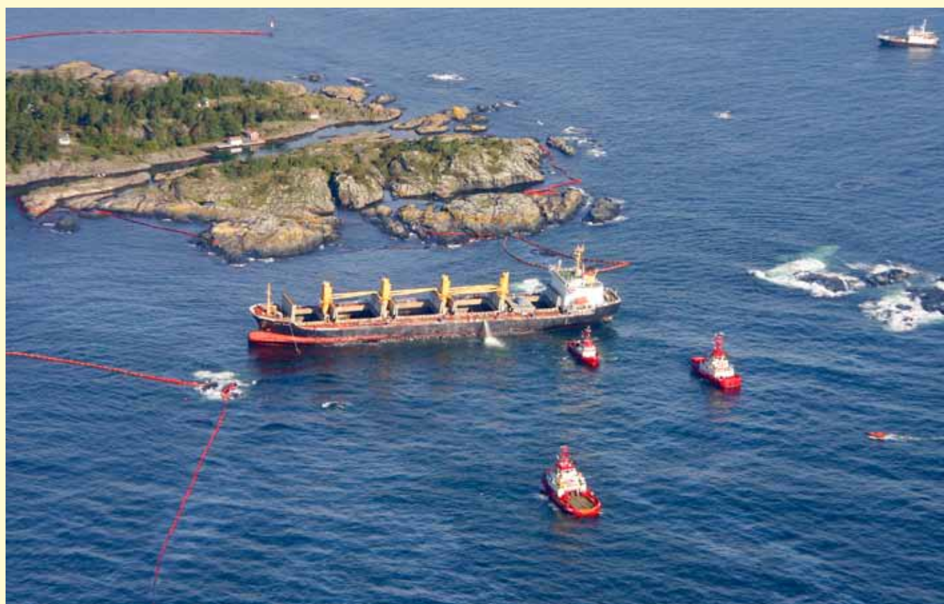
Bulk carrier "Full City" grounded on the rocks in stormy weather off the coast of Norway and was severely damaged. SMIT Salvage removed all heavy fuel oil from the tanks and, after several repairs, successfully refloated the vessel.
