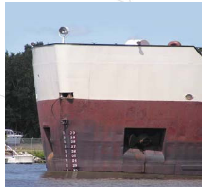
Lack of adequate dredging causes vessels to lightload to safely transit channels and ports.
