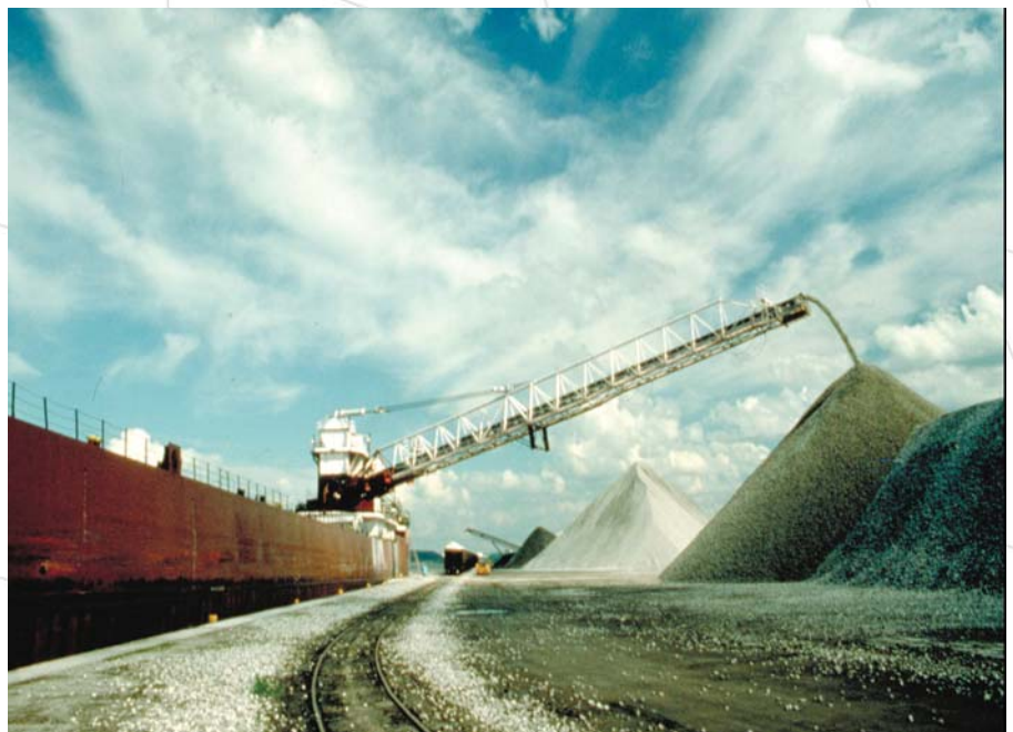
The GLNS supports jobs in many industries along the lakes. Here a self-unloading vessel discharges fluxstone in Duluth that will be used in the iron ore pelletizing process. The pellets then are shipped from Duluth to U.S. and Canadian steel mills throughout the Great Lakes region.
