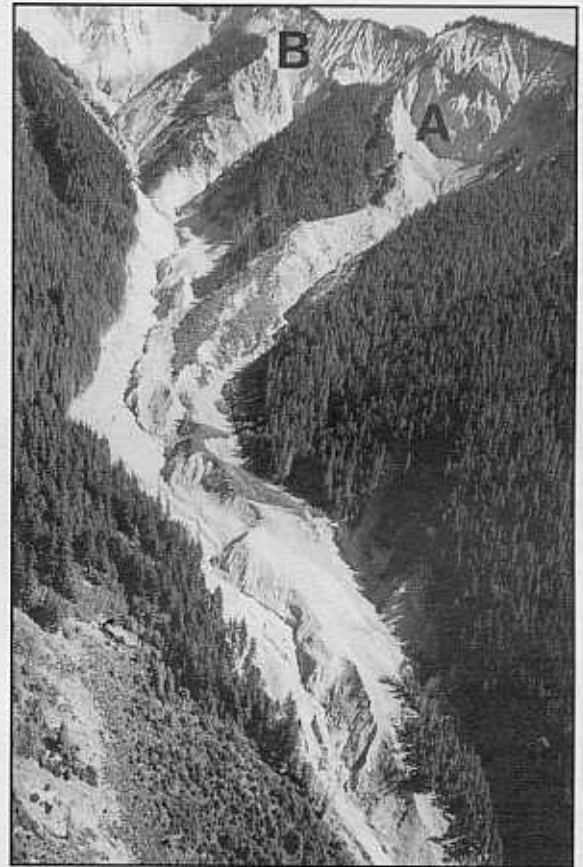
Figure 32. Aerial view of historic debris avalanches in Turbid Creek on the western slopes of Mount Cayley volcano; "A" is the source of the 1963 debris avalanche and "B" is the source of the 1984 event. Both landslides involved initial failure in Pleistocene pyroclastic rocks. This photograph, taken in 1985, shows the swath cut through the tree cover by the 1984 debris avalanche. GSC 204857-F
