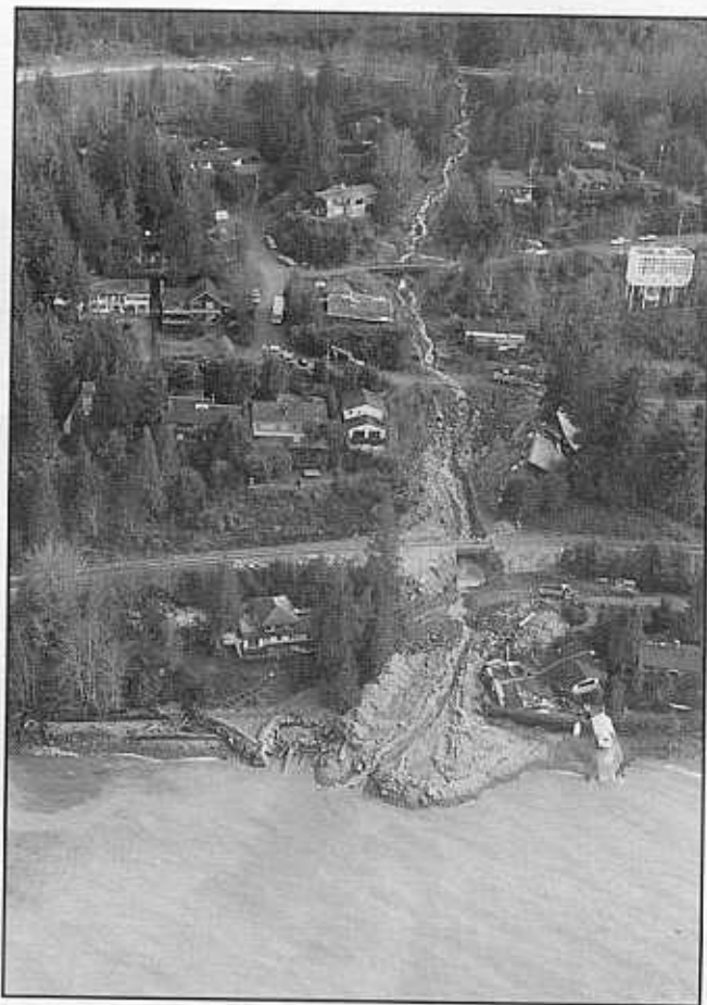
Figure 37. Alberta Creek debris flow, Lions Bay, which occurred on February 11, 1983. Note damaged buildings and bridges (photo courtesy of British Columbia Ministry of Highways and Communications).
