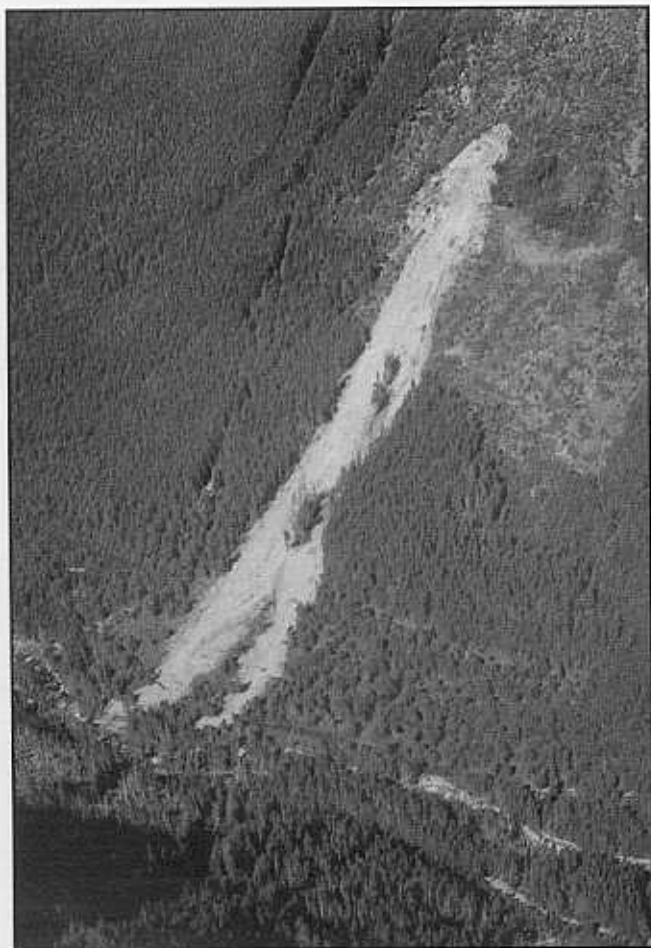
Figure 33. Debris avalanche (or open slope debris flow) which occurred in August 1991 as a result of heavy rains on north side of Britannia Creek, 4 km upstream of Britannia Beach. The landslide overran part of the abandoned townsite of Tunnel Camp. GSC 1994-492B
