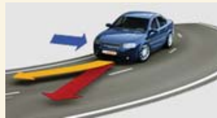
ESC "steers" the vehicle by intervening in the braking. The car is kept safely on track.
