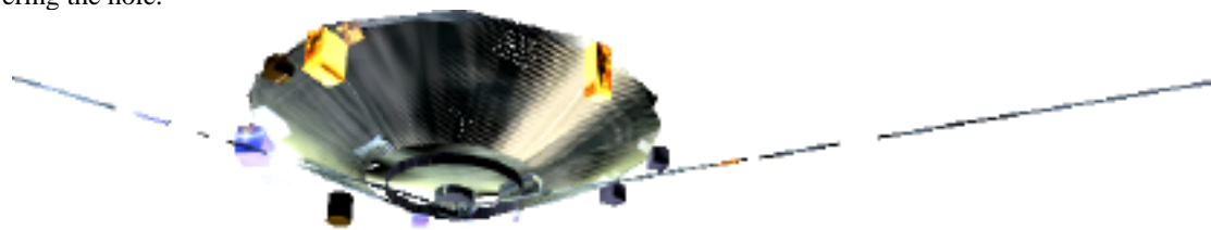
FIGURE 4. The spacecraft. The 2.7-m dish antenna serves as the main support structure. The instruments are attached near the rim of the antenna structure. The magnetometer boom and a dipole antenna for the plasma wave instrument are also visible
