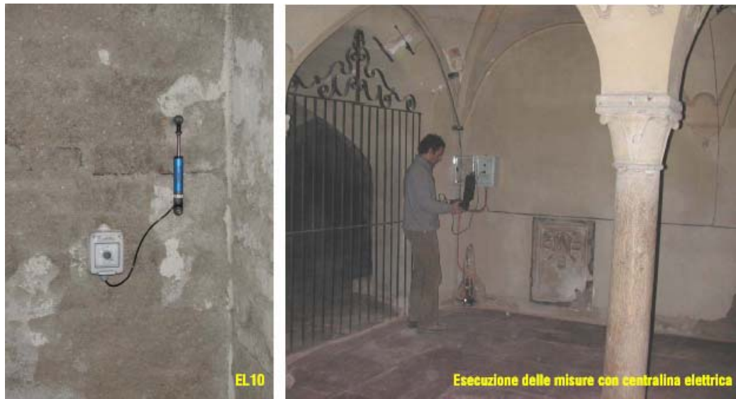
Figure 19: electric extensimeter EL10 and read-out of the displacements with the electronic switchboard
