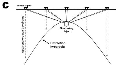
**Figure 8.** (a) Schematic representation of GPR survey configuration in cross-section. (b) Schematic representation of a single shaded GPR wiggle trace. (c) Discrete small features can generate GPR diffractions. The diffraction shape depends on the subsurface velocity above the scattering object. Migration of the profile involves collapsing the diffraction curves into a point.
