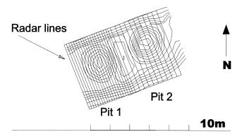
Figure 9. Diagram of GPR survey lines over two pits.
