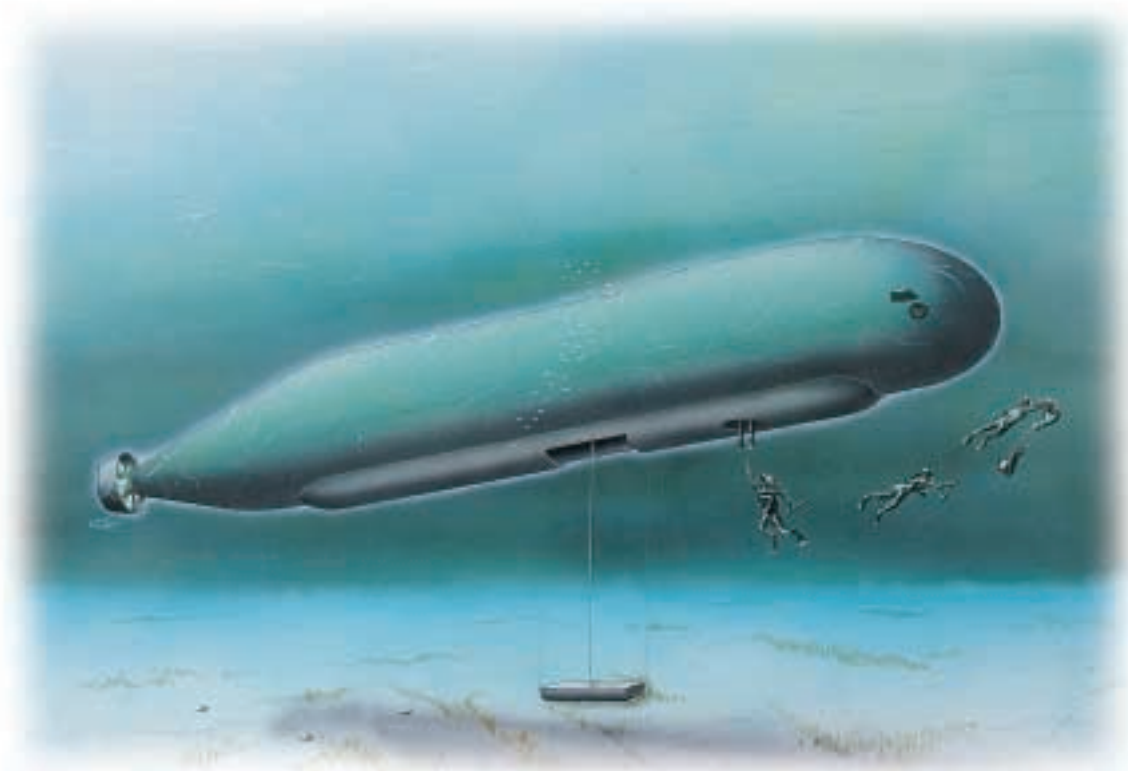
The Sea Dagger mini-submarine is of unique design, incorporating a replaceable centre section. Different modules can be used for the centre section, such as for transporting attack divers, for reconnaissance duties or for traditional attack missions.
