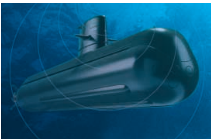
The hull design and various types of surface coatings minimize the risk of detection by active sonar.
