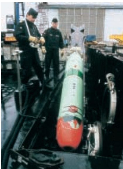
All that is needed ashore is a simple crane. The rest of the loading is handled by the system integrated into the submarine.
