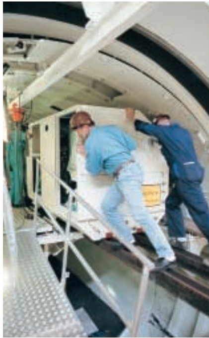
A Stirling unit being moved into the open hull section of a Gotland class submarine.
