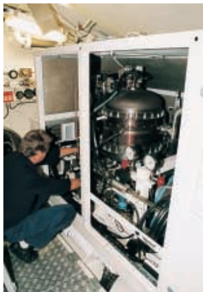
The Stirling AIP system is a compact, stand-alone unit that can be installed in existing submarines.
