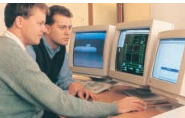
The Kockums SubTrainer is an advanced simulator for submarine manoeuvring. It can be used for training, for analysis of sea trials or for sessions aimed at trying out extreme and abnormal manoeuvres.
