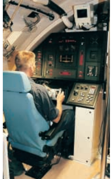
Due to one-man steering implemented by Kockums in 1963, manoeuvring the submarine below the surface has become much smoother and safer.
