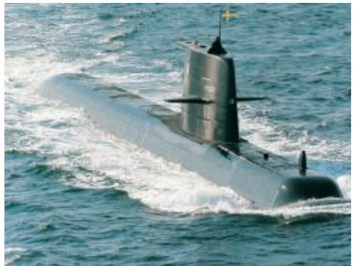
A submarine travelling on the surface or at periscope depth causes temperature changes and eddies in the surface water (wake) which can be detected by IR sensors or radar.
