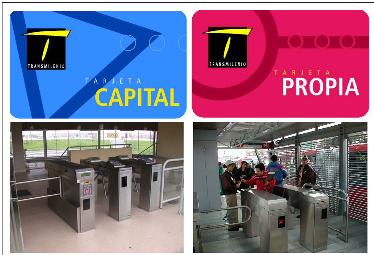
FIGURE 2.11 – TransMilenio’s Electronic Toll Collection System
