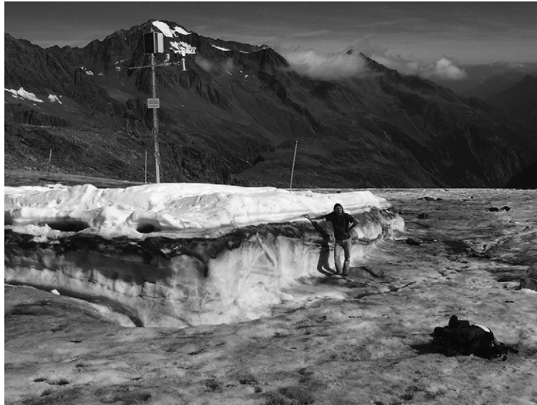
Fig. 10. Cover test area Schaufelferner after the removal of the geotextiles at the end of the ablation period on 16 September 2005. Natural glacier ice ablation ( 900 \text{ kgm}^{-2} ) was completely stopped and 315 \text{ kgm}^{-2} of winter snow were preserved over the ablation period.
