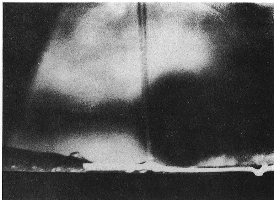
Fig. 6. Photomicrograph of light-pipe area with limiting volume of solution ( \approx 1.5 nl) across gap.
