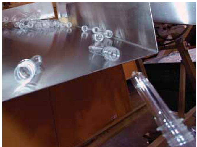
PET bottle pre-forms are loaded into a bottle-blowing machine.
