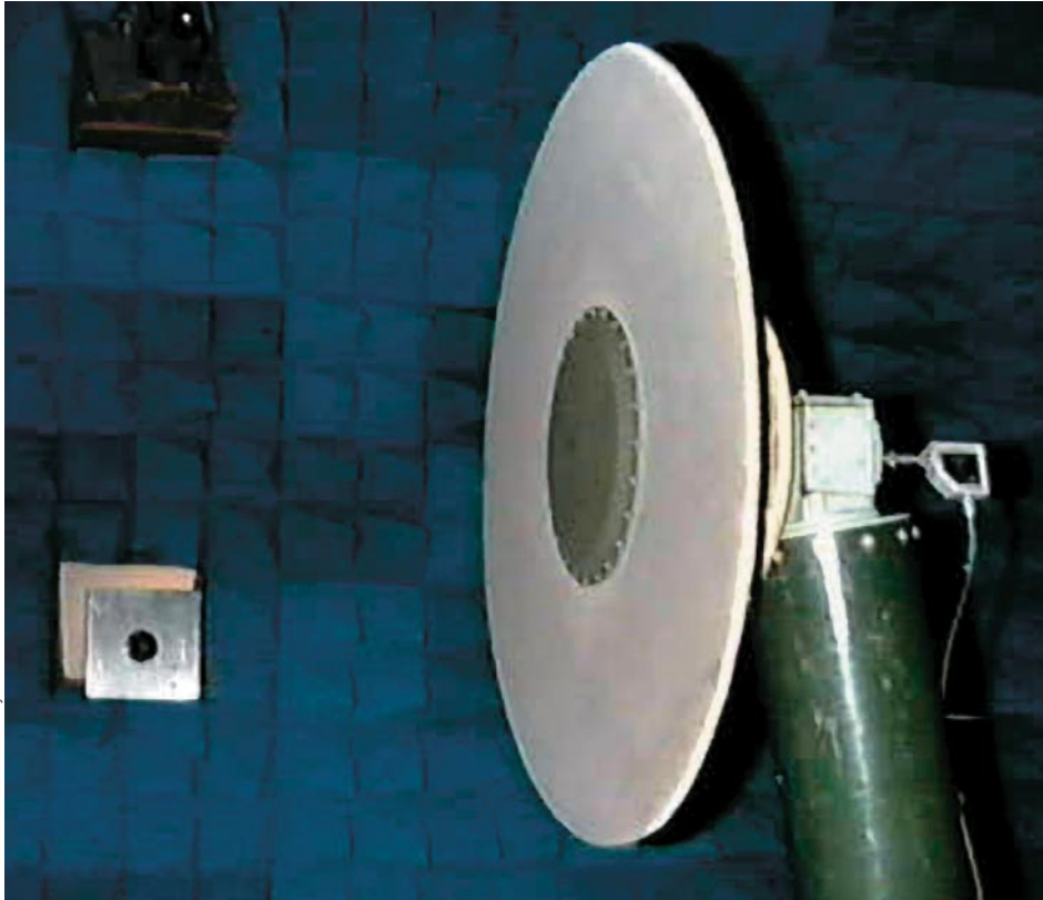
A jam-resistant GPS antenna undergoes testing at the Air Force Research Laboratory.
