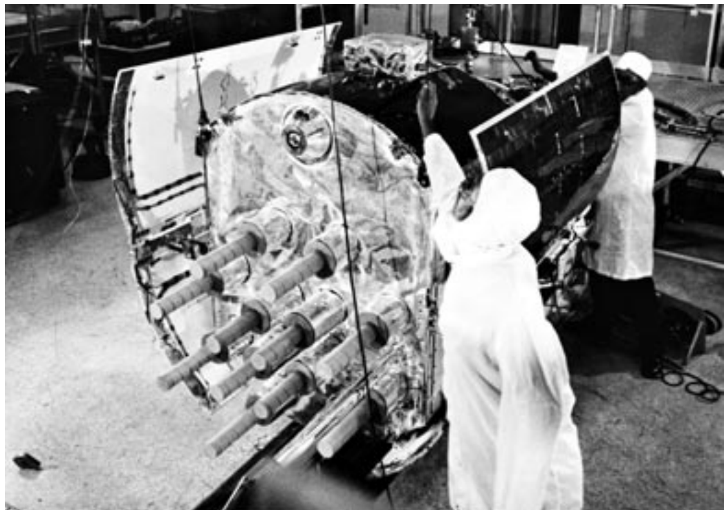
Weight and balance tests of the third prototype satellite in the Navstar/GPS constellation are conducted prior to its launch from Vandenberg Air Force Base.
