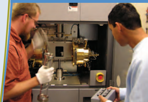
Students and postdocs work with MSU's optical-image furnace to grow single crystals of advanced materials
