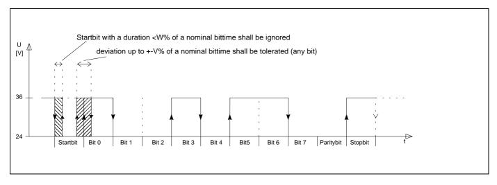
Fig. 5: Minimum duration start element (Receive)
