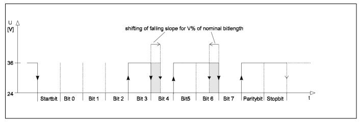
Fig. 3: Practical receive margin (example for two falling slopes)
