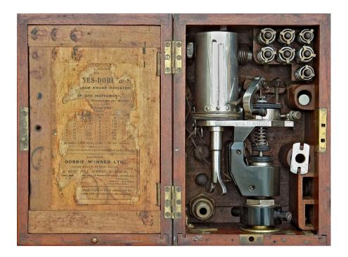
**Plate 0–5.** This Dobbie McInnes Design No. 1A indicator, no. 16813L dating from *c*. 1917, is known to have been used by a Surveyor employed by the British Engine Boiler & Electrical Insurance Co. Ltd. Unlike standard Design No. 1A instruments, which have the distinctively arched tracer bar, the 'L' type has a straight arm and a large drum intended for use with Richards-type paper. *John Walter collection*.
