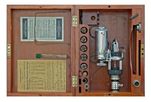
**Plate 0–7.** Dobbie McInnes Ltd introduced the Design No. 4 indicator, a refinement of the old No. 1A, shortly after the end of the Second World War. This example, no. 45074, probably dates from 1948. British-made indicators customarily lacked the wide range of accessories offered with the German rivals. *Museum of Making collection*.
