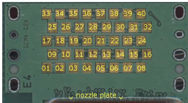
Fig. 19 ip2000 printhead contact pin layout
