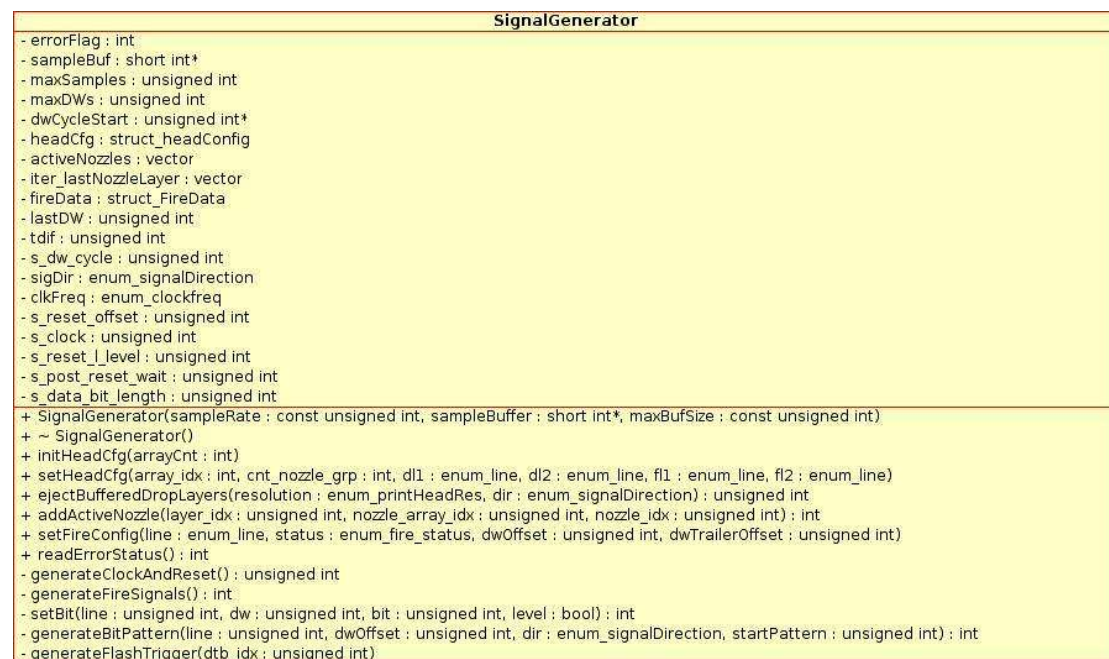
Fig. 41 UML diagram of SignalGenerator class. Created with Umbrello [54].
