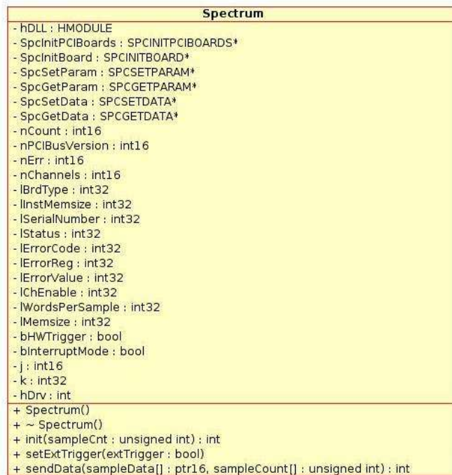
Fig. 42 UML diagram of Spectrum class. Created with Umbrello [54].
