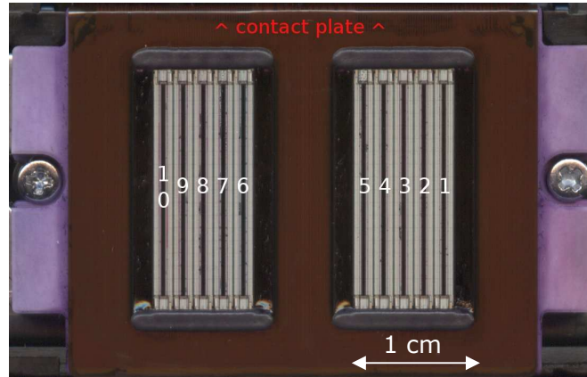
Fig. 20 ip8500 printhead nozzle plate layout
