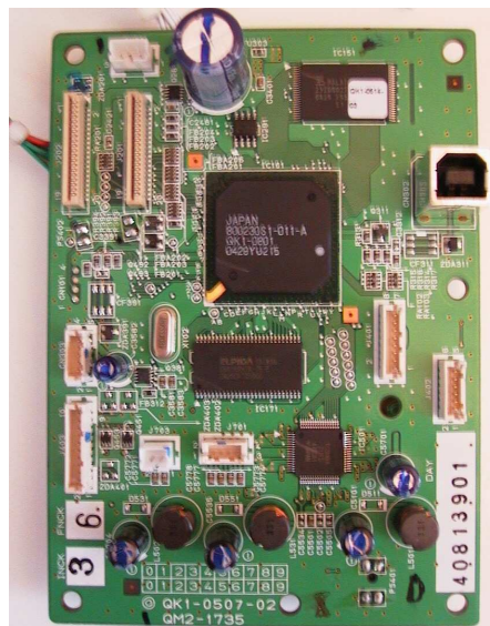
Fig. 18 ip2000 printer controller board
