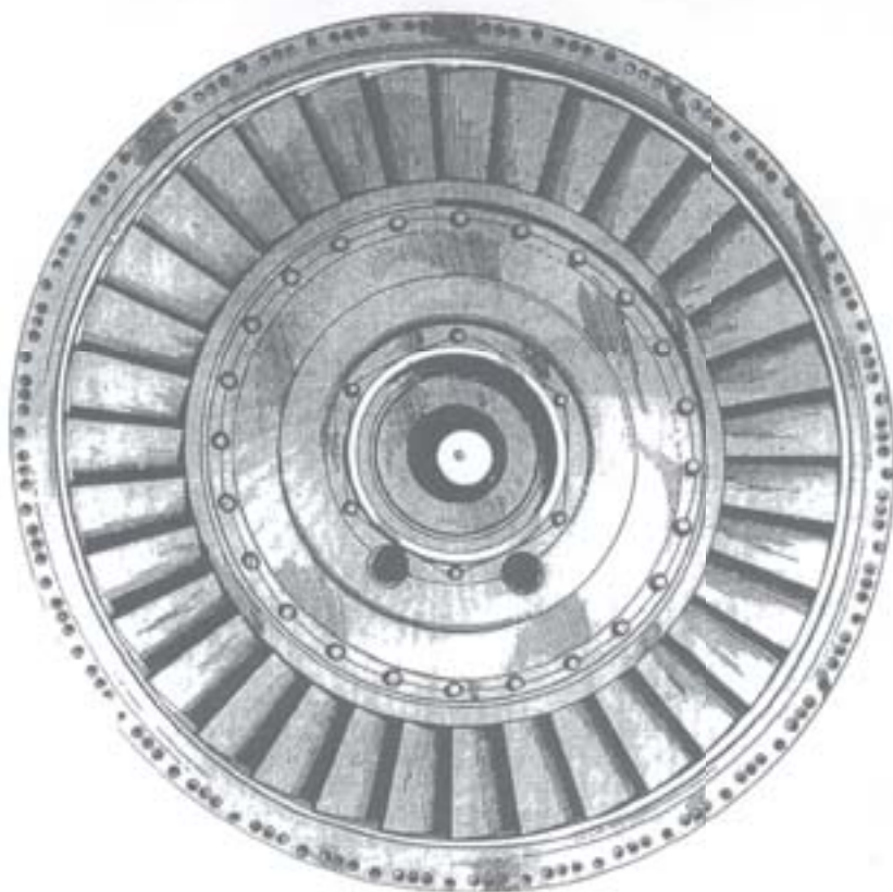
Front view of turbine nozzle assembly showing rear turbine bearing and diaphragm plates in place. Cooling air enters two holes seen just below bearing, goes up between diaphragm plates and through nozzle roots, then out through openings in trailing edges. Note 36 bolt holes (in outer rear flange) for attaching assembly to combustion chamber casing, also 36 series-of-three holes for carrying exhaust system cooling air.
