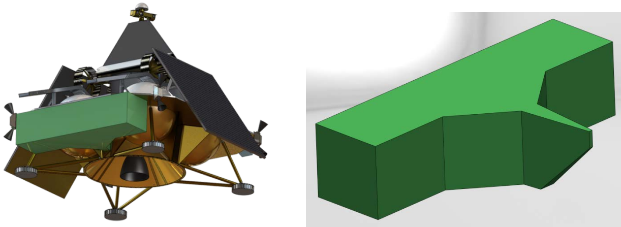
Figure 4-2: Thermally controlled payload volumes exist under the deck on the two edges with ramps. Iso view shows detail of the shape.
