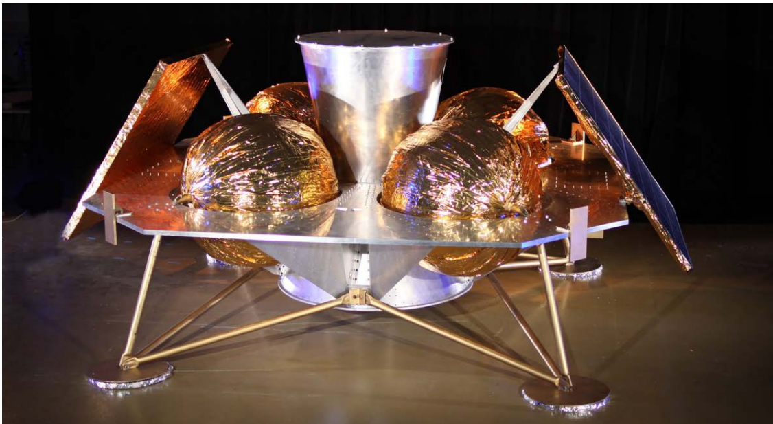
Figure 3-2: Lander structure prior to addition of egress ramps and upgraded energy-absorbing legs
