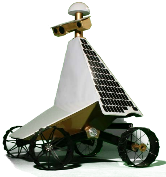
Figure 2-4: Prototype robot showing four-facet solar panel configuration
