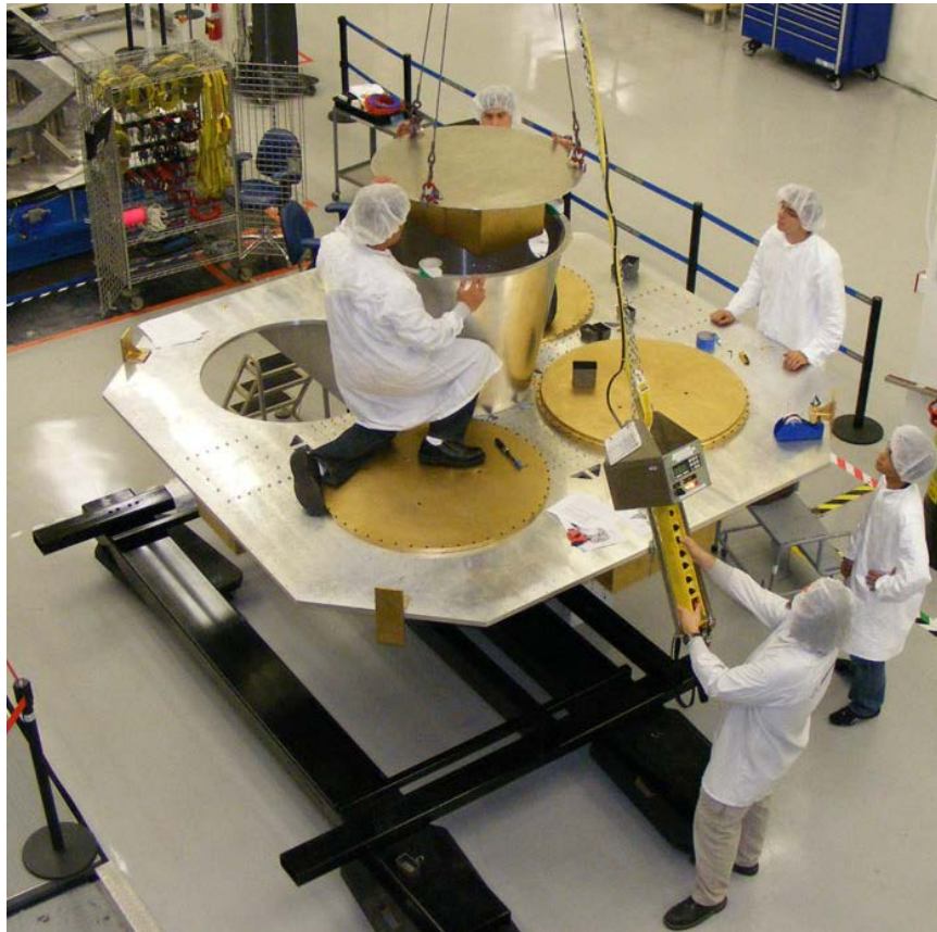
Figure 4-10: Astrobotic's lander structure passed shake table tests for acceleration and with confirmation that first lateral and first axial modes of vibration are sufficiently higher than Falcon 9 requirements
