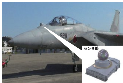
IRST装置 Infra-Red Search and Track System
