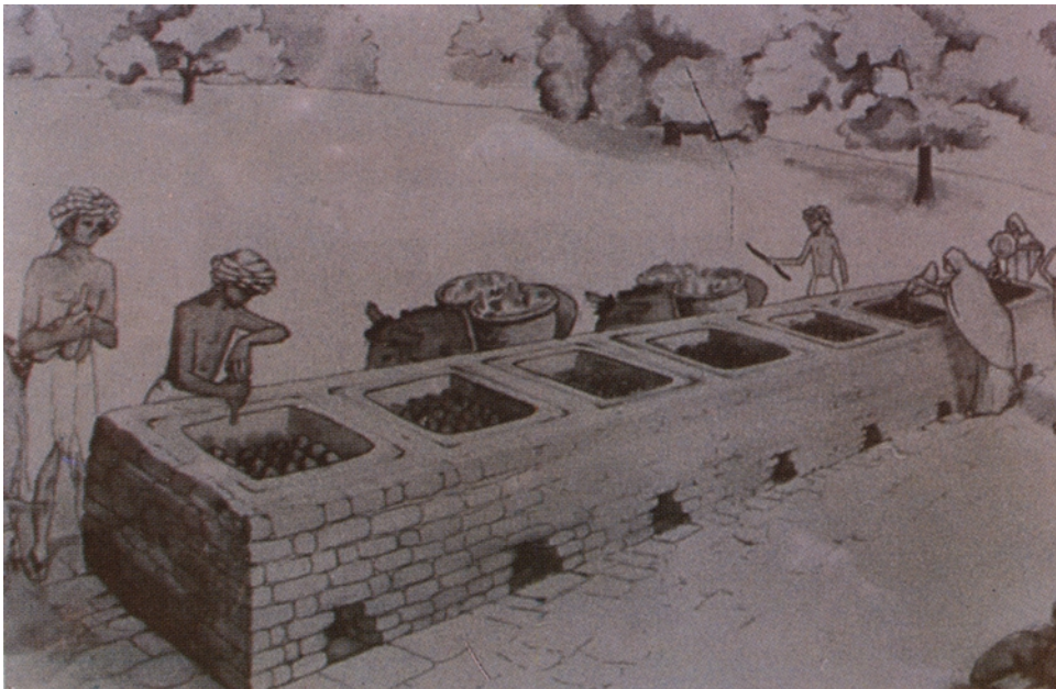
Fig. 10 An artist's view of the working of the process of zinc smelting furnace
