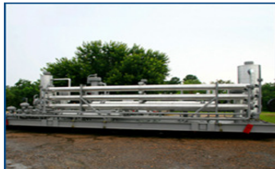
Figure 23: Membrane technology for CO 2 removal [9.25]
