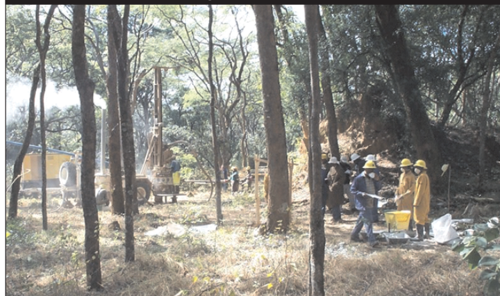
REVERSE CIRCULATION DRILLING ON THE LUBEMBE PROJECT SHOWING THE DENSE WOODLAND VEGETATION OF THE AREA
