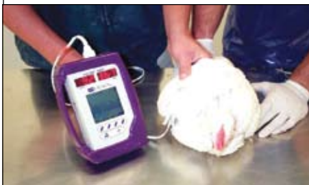
Blood oximetry provides a measure of the cardiovascular health of birds, helping to reduce the incidence of ascites.
