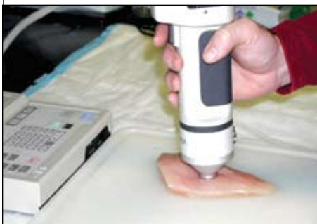
Colorimetry is used to assess meat colour, helping to achieve uniform colour in chicken parts.
