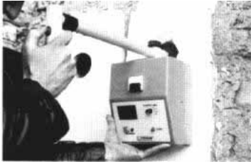
Figure 10. Neutron-based instrument for moisture measurement.
