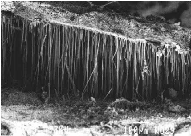
Figure 13, bottom right. Paint layer lifted by nitronatrite whiskers, thinning out toward their base on the substrate from which they have grown.
