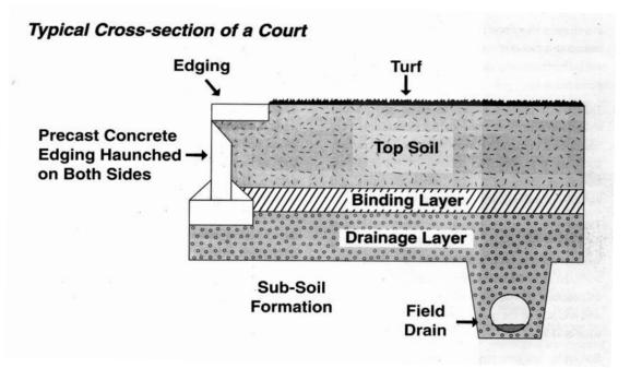
(2 inches) depths at a time, with each layer being heeled-in, raked, levelled, then heeled and raked again. Such a process is clearly very slow and labour-intensive, but this careful attention to detail is important to ensure a firm surface and to avoid any future unevenness through sinkage.
