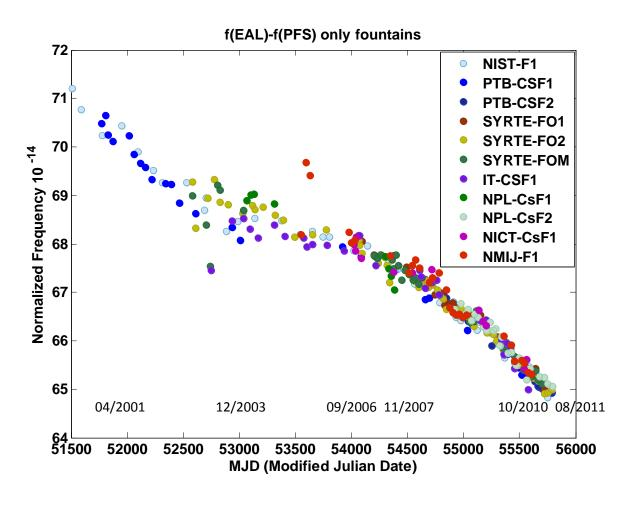
A drift has been observed in the last years between the « free » time scale EAL and the primary frequency standards. Improvement of the algorithm of calculation of TAI/UTC at the BIPM with a new model for the clock frequency prediction is stopping the drift.
