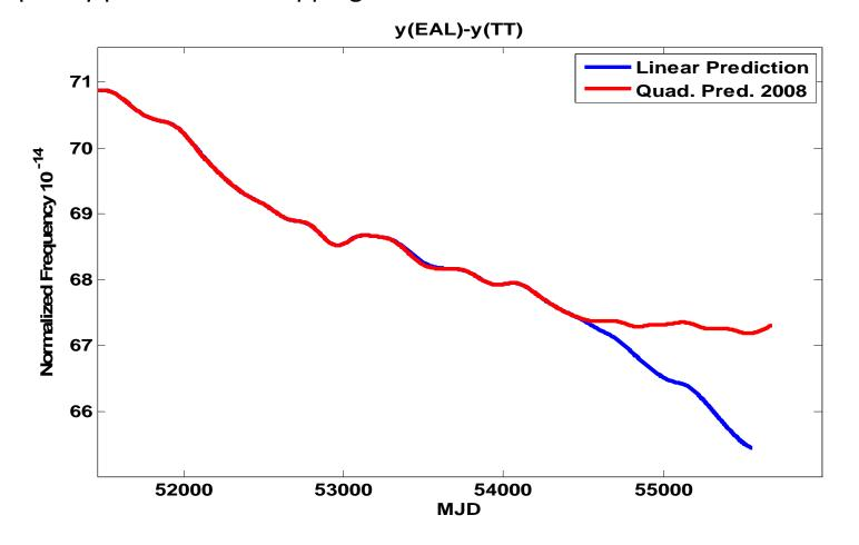
Improvement of the frequency stability of TAI/UTC with the new clock frequency prediction model
