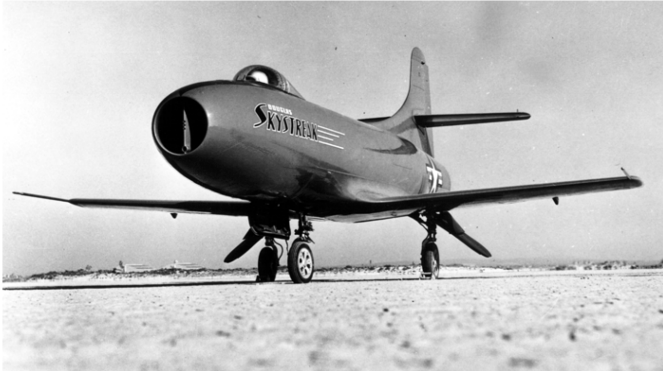
Photo 3.4—The Douglas D-558-1 Skystreak took part in an experimental Navy high-speed test program beginning in May 1947. Unlike its contemporary, the Bell X-1, the Skystreak was incapable of breaking the sound barrier.
