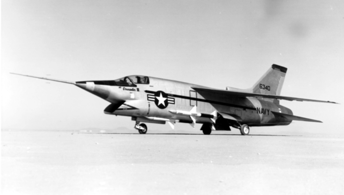
Photo 3.11—Vought developed the all-new F8U-3 Crusader III in the late 1950s to compete with the McDonnell F4H-1 Phantom II for selection as the Navy's next carrier-based fleet air-defense fighter. Only three examples of the Mach 2.5 fighter flew, since the Navy canceled the program after selection of the Phantom in late 1958.
