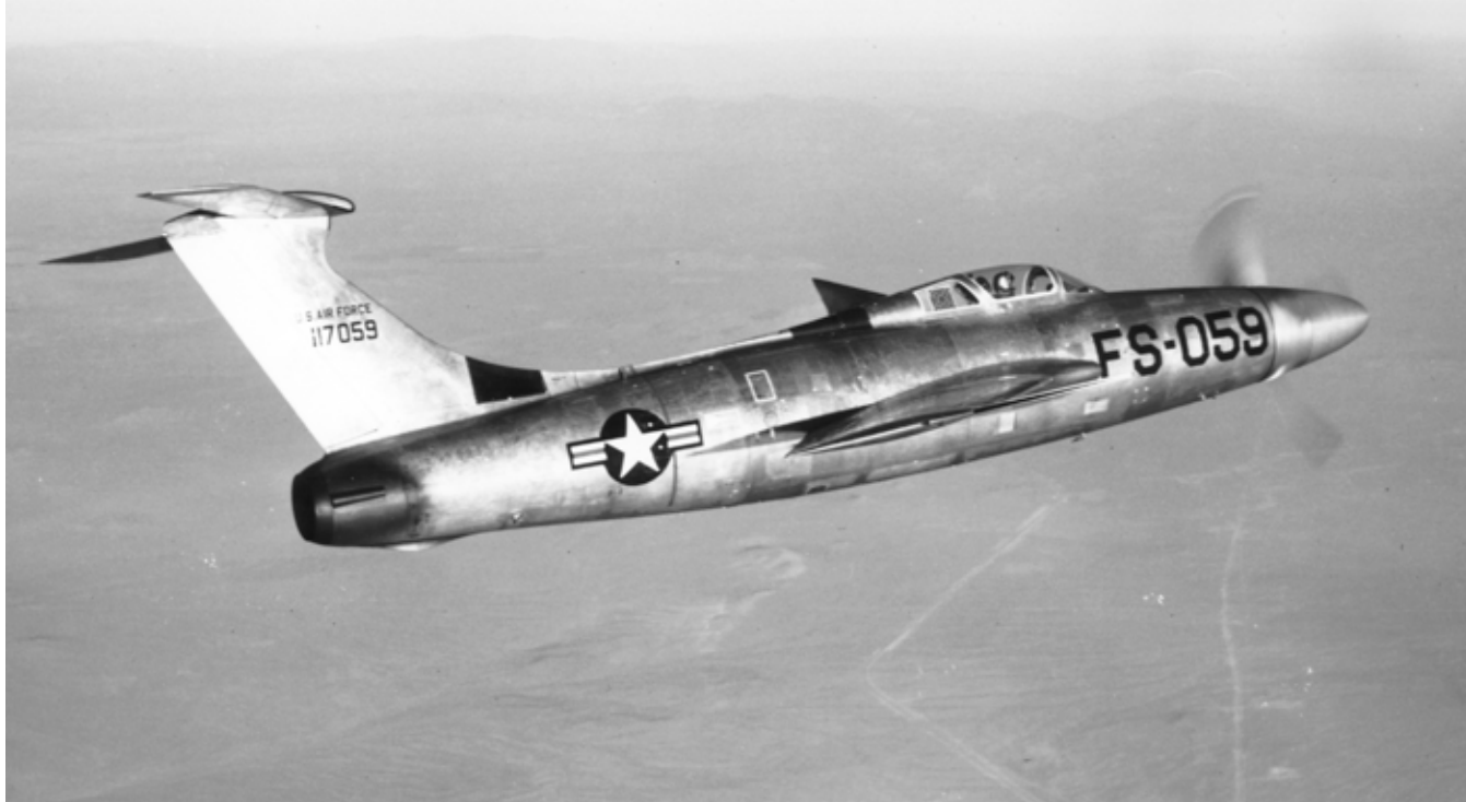
Photo 2.10—The Republic XF-84H investigated the use of turboprops to enhance short-takeoff capabilities for fighter bombers. First flight took place July 10, 1955.
