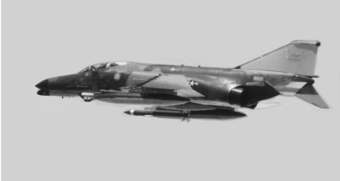
Photo 4.1—The McDonnell F-4 Phantom has been characterized as the most significant and successful Western fighter of the 1960s. First flown as a Navy fighter in May 1958, the F-4 was eventually procured in large numbers by the U.S. Air Force and several foreign air forces.
