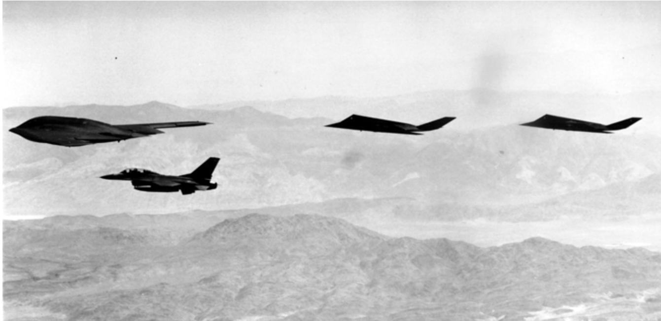
Photo 6.2—America's first-generation stealth combat aircraft, the Northrop B-2 bomber and Lockheed F-117 attack fighters, accompanied by a Lockheed (formerly General Dynamics) F-16 in the foreground.
