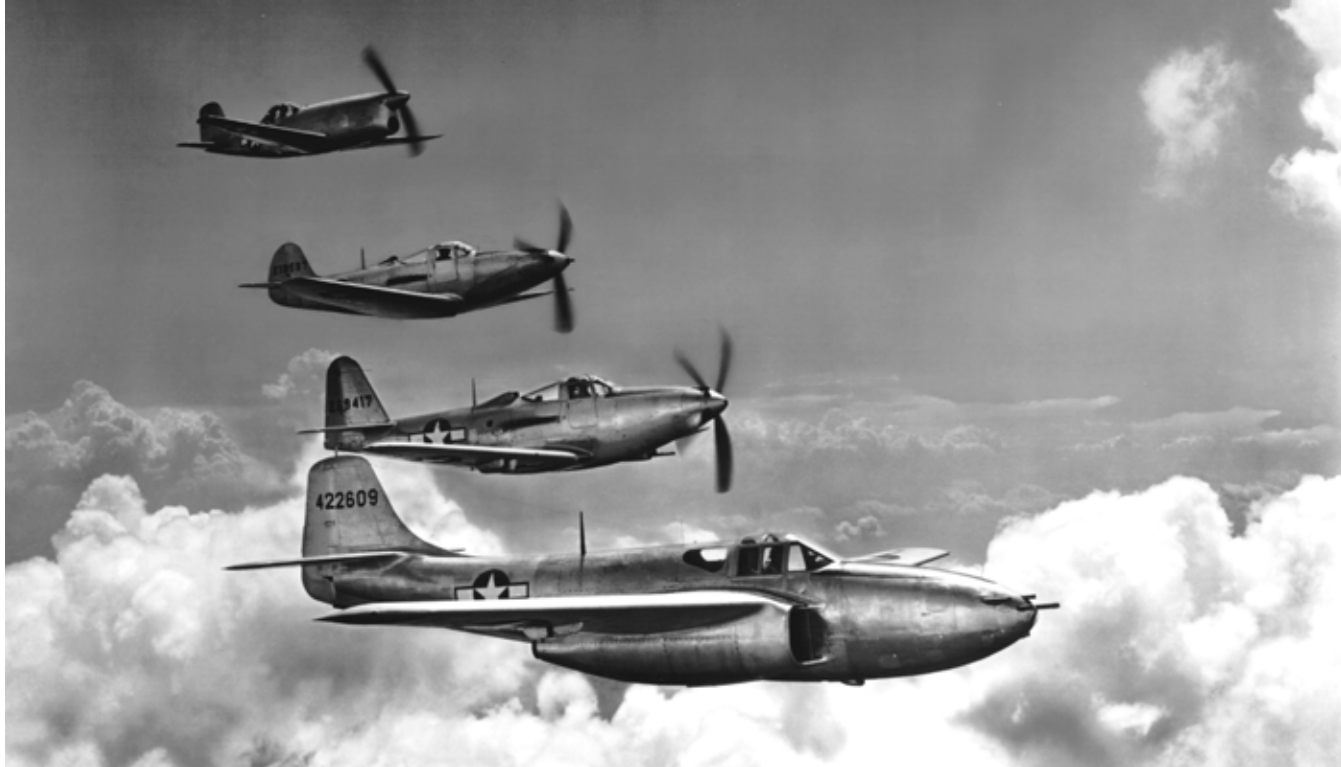
Photo 2.3—The Bell P-59 Airacomet (foreground) was America's first operational jet fighter. First flown in October 1942, the P-59 proved to be a disappointment because of its relatively slow top speed. Behind the P-59 (front to back) can be seen three other World War II Bell fighters: the P-63 King Cobra, the famous P-39 Airacobra, and the little-known lightweight XP-77.
