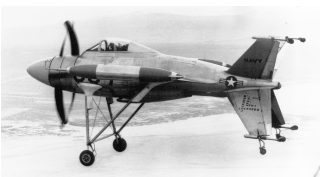
Photo 2.11—The turboprop-powered Lockheed XFV-1, pictured here, competed in 1954 and 1955 with the Convair XFY-1 to provide a tail-sitting vertical-takeoff fighter for the Navy. Both prototypes proved unsuccessful.
