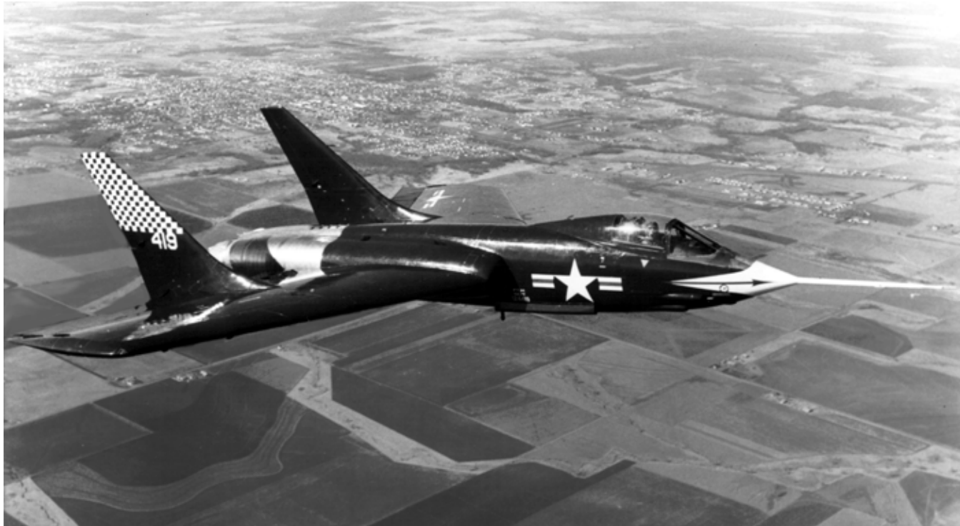
Photo 2.14—A variant of the Vought F7U-1 Cutlass. First flying in 1948, this highly unorthodox fighter design experienced numerous developmental problems. Vought eventually redesigned the fighter as the F7U-3 Cutlass.
