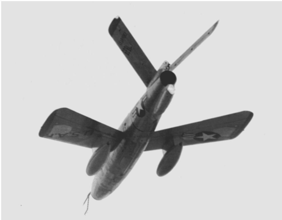
Photo 2.9—The innovative Republic XF-91 Thunderceptor, which first flew in May 1949, was conceived as a high-altitude interceptor. In late 1951, the Air Force canceled further development of the XF-91 in favor of the Convair F-102.
