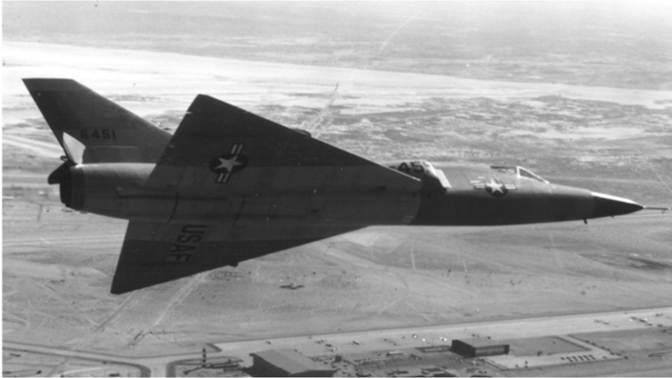
Photo 3.2—The Convair F-106A Delta Dart was the final outcome of the “Ultimate Fighter” competition of the early 1950s. Originally viewed as a modification of the Convair F-102B Delta Dagger, so many changes were required to overcome the shortcomings of the F-102B that the upgraded aircraft was awarded the new designation of F-106A.
