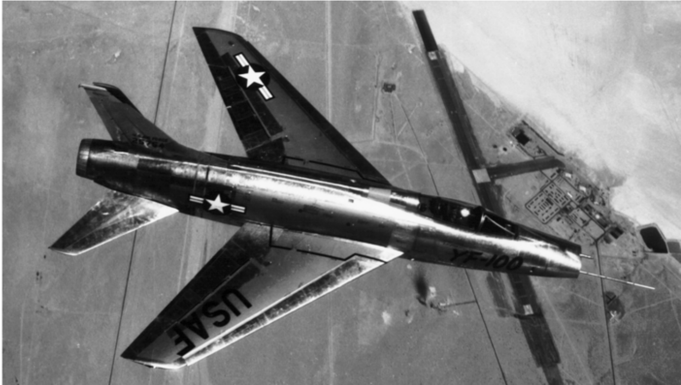
Photo 3.1—The North American F-100 Super Sabre, first flown in May 1953, grew out of a company-funded project to become the first fighter to achieve sustained, level supersonic flight.
