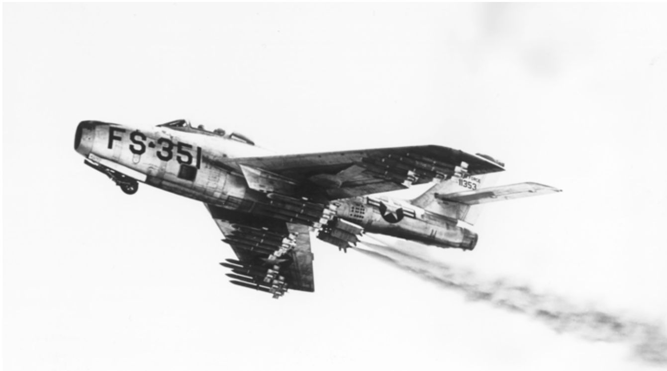
Photo 2.12—The Republic F-84F Thunderstreak was a greatly modified swept-wing version of the F-84E that was widely procured by European allies in the 1950s, as well as by the U.S. Air Force.
