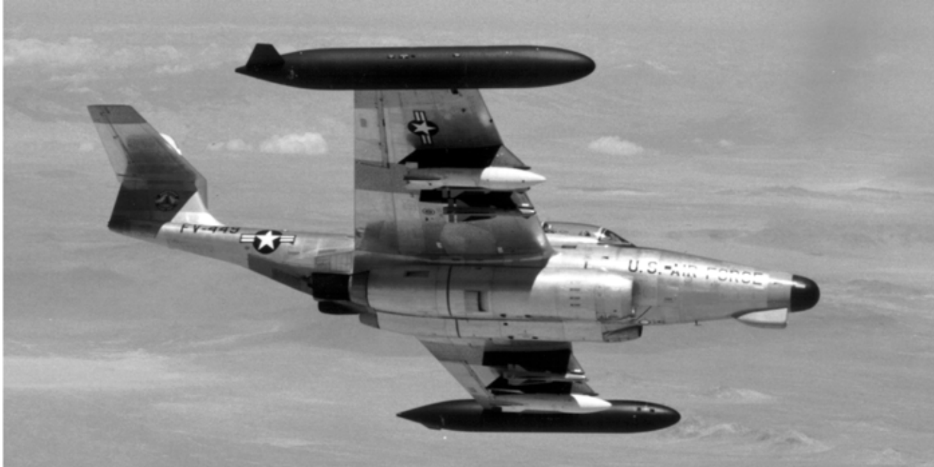
Photo 2.8—The Northrop F-89J Scorpion, as shown here, carried unguided AIR-2A Genie air-to-air missiles armed with nuclear warheads. First flown in August 1948, the F-89 was the last Northrop combat aircraft procured by the Air Force before the stealth era.
