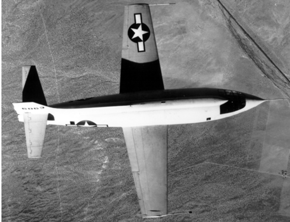
Photo 3.3—The famous Bell X-1 was developed by the Air Force and NACA to investigate supersonic flight. On October 14, 1947, an X-1 piloted by Capt. Charles “Chuck” Yeager became the first aircraft to exceed the speed of sound.
