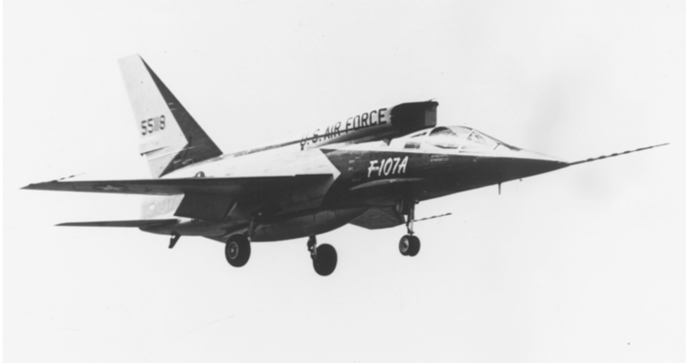
Photo 3.8—Featuring an innovative air intake position above and behind the cockpit, the North American YF-107A flew in competition with the Republic F-105 Thunderchief for selection as a supersonic deep-penetration nuclear strike fighter. The YF-107A was canceled in 1956 after selection of the Thunderchief. The YF-107A was North American's last flying fighter design.
