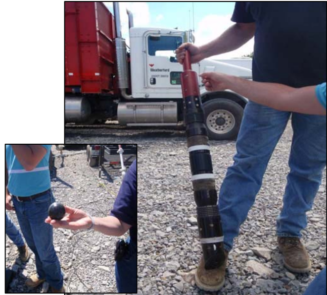
A Ball and Ball Packer (Pennsylvania Marcellus Shale) Source: ALL Consulting 2008
