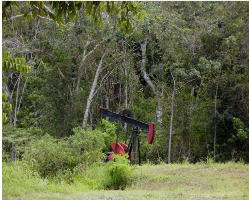
Figure 3: Pumping jack belonging to Soca Petroleum Limited in operation in Trinidad. Source: Jean-Jacques Limage.
