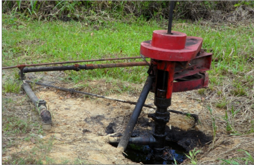
Figure 4: Economical field development: a refitted cavitation pump at Morne Diablo.
