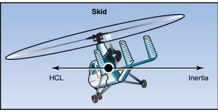
Figure 20-9. During a skid, inertia exceeds the HCL. To reestablish equilibrium, increase the bank angle or reduce the rate of turn by applying rudder pedal. You may also use a combination of these two corrections.
