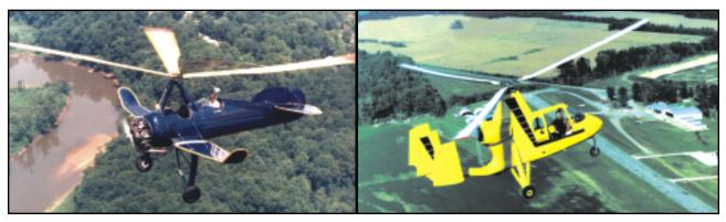
Figure 15-1. The gyroplane may have wings, be either tractor or pusher configured, and could be turbine or propeller powered. Pictured are the Pitcairn PCA-2 Autogyro (left) and the Air & Space 18A gyroplane.
