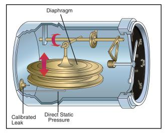
Figure 12-4. Although the sealed case and diaphragm are both connected to the static port, the air inside the case is restricted through a calibrated leak. When the pressures are equal, the needle reads zero. As you climb or descend, the pressure inside the diaphragm instantly changes, and the needle registers a change in vertical direction. When the pressure differential stabilizes at a definite ratio, the needle registers the rate of altitude change.
