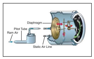
Figure 12-2. Ram air pressure from the pitot tube is directed to a diaphragm inside the airspeed indicator. The airtight case is vented to the static port. As the diaphragm expands or contracts, a mechanical linkage moves the needle on the face of the indicator.
