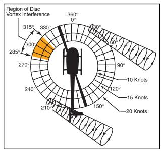
Figure 11-10. Main rotor disc vortex interference.
