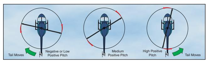
Figure 4-6. Tail rotor pitch angle and thrust in relation to pedal positions during cruising flight.
