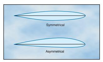
Figure 2-2. The upper and lower curvatures are the same on a symmetrical airfoil and vary on an asymmetrical airfoil.
