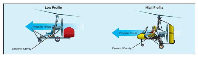
Figure 16-9. A gyroplane which has the propeller thrust line above the center of gravity is often referred to as a low profile gyroplane. One that has the propeller thrust line below or at the CG is considered a high profile gyroplane.
