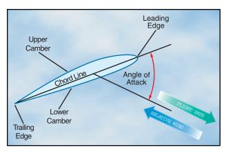
Figure 2-3. Aerodynamic terms of an airfoil.
