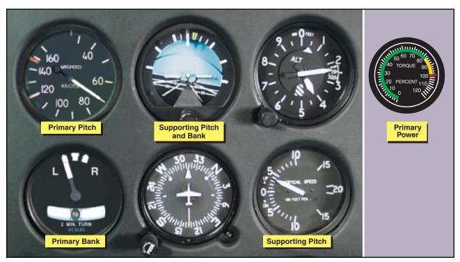
Figure 12-21. Flight instrument indications for a stabilized left climbing turn at a constant airspeed.
