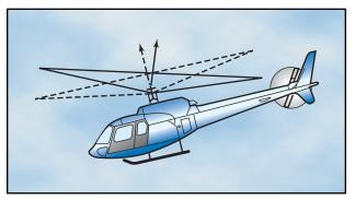
Figure 3-16. To compensate for blowback, you must move the cyclic forward. Blowback is more pronounced with higher airspeeds.
