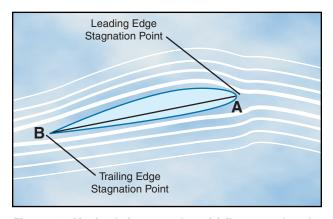
Figure 2-8. Air circulation around an airfoil occurs when the front stagnation point is below the leading edge and the aft stagnation point is beyond the trailing edge.
