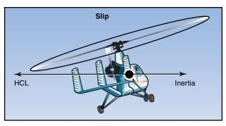
Figure 20-8. During a slip, the rate of turn is too slow for the angle of bank used, and the horizontal component of lift (HCL) exceeds inertia. You can reestablish equilibrium by decreasing the angle of bank, increasing the rate of turn by applying rudder pedal, or a combination of the two.
