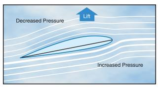
Figure 2-10. Lift is produced when there is decreased pressure above and increased pressure below an airfoil.
