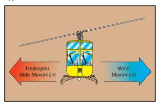
Figure 9-9. During a slip, the rotor disc is tilted into the wind.
