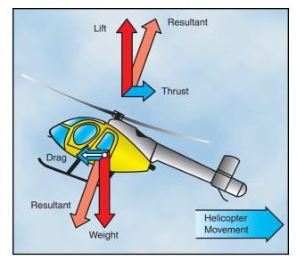
Figure 3-18. Forces acting on the helicopter during rearward flight.
