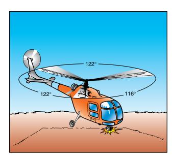
Figure 11-5. Hard contact with the ground can send a shock wave to the main rotor head, resulting in the blades of a three-bladed rotor system moving from their normal 120° relationship to each other. This could result in something like 122°, 122°, and 116° between blades. When one of the other landing gear strikes the surface, the unbalanced condition could be further aggravated.
