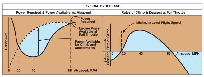
Figure 20-13. The low point on the power required curve is the speed that the gyroplane can fly while using the least amount of power, and is also the speed that will result in a minimum sink rate in a power-off glide.
