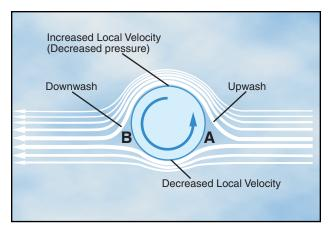
Figure 2-7. Magnus Effect is a lifting force produced when a rotating cylinder produces a pressure differential. This is the same effect that makes a baseball curve or a golf ball slice.
