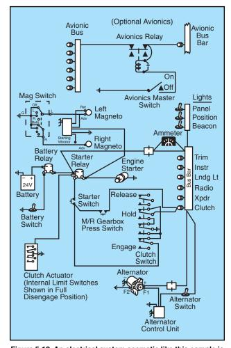
Figure 5-12. An electrical system scematic like this sample is included in most POHs. Notice that the various bus bar accessories are protected by circuit breakers. However, you should still make sure all electrical equipment is turned off before you start the engine. This protects sensitive components, particularly the radios, from damage which may be caused by random voltages generated during the starting process.
