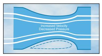
Figure 2-9. The upper surface of an airfoil is similar to the constriction in a venturi tube.
