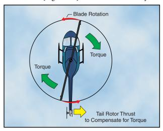
Figure 1-3. The antitorque rotor produces thrust to oppose torque and helps prevent the helicopter from turning in the opposite direction of the main rotor.
