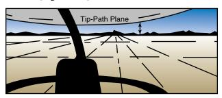
Figure 9-11. You can maintain a straight-and-level attitude by keeping the tip-path plane parallel to and a constant distance above or below the natural horizon. For any given airspeed, this distance remains the same as long as you sit in the same position in the same type of aircraft.
