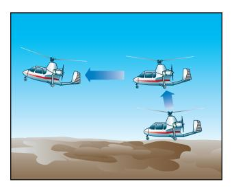
Figure 20-5. During a jump takeoff, excess rotor inertia is used to lift the gyroplane nearly vertical, where it is then accelerated through minimum level flight speed.
