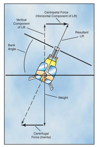
Figure 3-19. The horizontal component of lift accelerates the helicopter toward the center of the turn.
