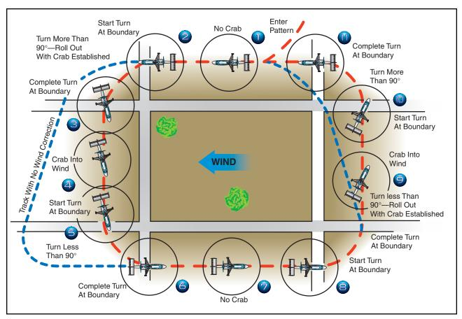
Figure 20-10. Rectangular course. The numbered positions in the text refer to the numbers in this illustration.
