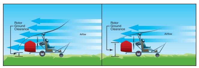
Figure 20-3. Decreasing the rotor disc angle of attack with forward cyclic can reduce the excessive amount of airflow causing the blade flap. This also allows greater clearance between the rotor blades and the surface behind the gyroplane, minimizing the chances of a blade striking the ground.
