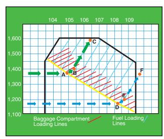
Figure 7-6. Loading chart illustrating the solution to sample problems 1 and 2.
