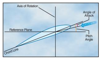
Figure 2-6. Angle of attack may be greater than, less than, or the same as the pitch angle.
