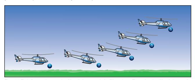
Figure 9-8. The helicopter takes several positions during a normal takeoff from a hover. The numbered positions in the text refer to the numbers in this illustration.
