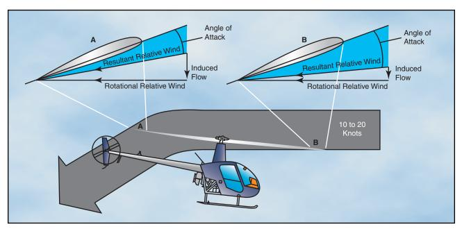
Figure 3-13. A helicopter in forward flight, or hovering with a headwind or crosswind, has more molecules of air entering the aft portion of the rotor blade. Therefore, the angle of attack is less and the induced flow is greater at the rear of the rotor disc.
