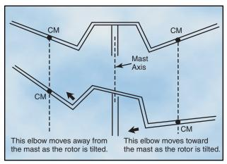
Figure 3-6. Because of the underslung rotor, the center of mass remains approximately the same distance from the mast after the rotor is tilted.
