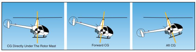
Figure 7-1. The location of the center of gravity strongly influences how the helicopter handles.
