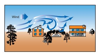
Figure 10-8. If the wind velocity is 10 knots or greater, you should expect updrafts on the windward side and downdrafts on the lee side of obstacles. You should plan the approach with these factors in mind, but be ready to alter your plans if the wind speed or direction changes.
