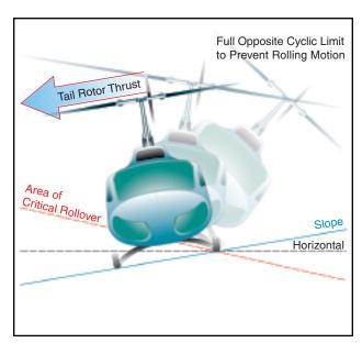
Figure 11-8. Downslope rolling motion.
