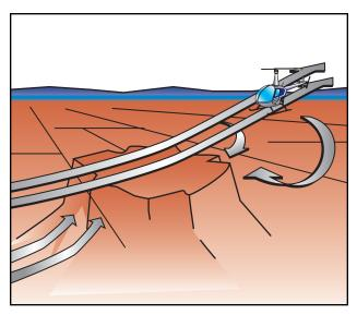
Figure 10-9. When flying an approach to a pinnacle or ridgeline, avoid the areas where downdrafts are present, especially when excess power is limited. If you encounter downdrafts, it may become necessary to make an immediate turn away from the pinnacle to avoid being forced into the rising terrain.
