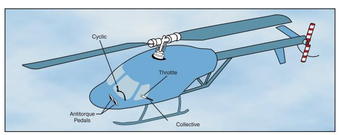
Figure 1-7. Location of flight controls.
