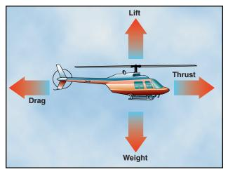
Figure 2-1. Four forces acting on a helicopter in forward flight.
