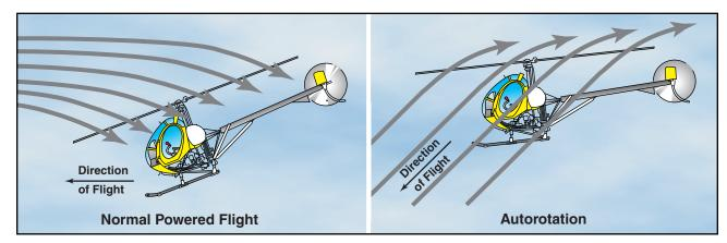
Figure 3-20. During an autorotation, the upward flow of relative wind permits the main rotor blades to rotate at their normal speed. In effect, the blades are "gliding" in their rotational plane.
