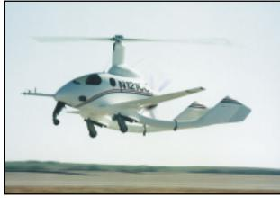
Figure 15-3. The CarterCopter uses wings to enhance performance.
