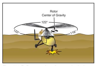
Figure 21-2. Taxiing on rough terrain can send a shock wave to the rotor system, resulting in the blades of a three-bladed rotor system moving from their normal 120° relationship to each other.
