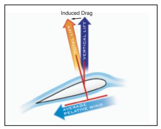
Figure 2-13. The formation of induced drag is associated with the downward deflection of the airstream near the rotor blade.
