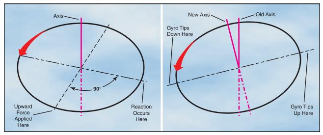
Figure 3-8. Gyroscopic precession principle—when a force is applied to a spinning gyro, the maximum reaction occurs approximately 90° later in the direction of rotation.
