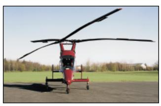
Figure 1-2. Helicopters can have a single main rotor or a dual rotor system.
