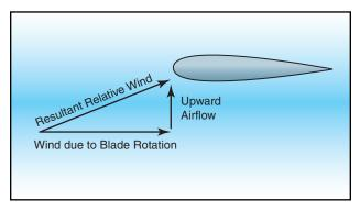
Figure 16-2. In a vertical autorotation, the wind from the rotation of the blade combines with the upward airflow to produce the resultant relative wind striking the airfoil.
