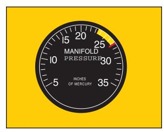
Figure 6-5. A manifold pressure gauge is commonly used with piston-powered aircraft.
