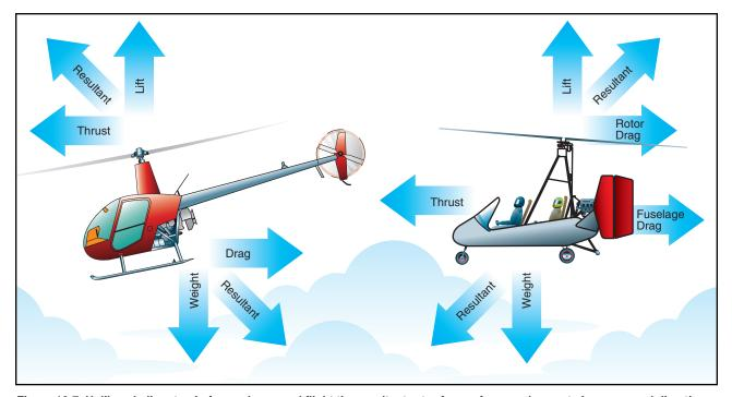
Figure 16-7. Unlike a helicopter, in forward powered flight the resultant rotor force of a gyroplane acts in a rearward direction.
