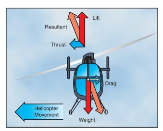
Figure 3-17. Forces acting on the helicopter during sideward flight.
