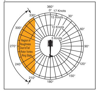
Figure 11-12. Tail rotor vortex ring state.
