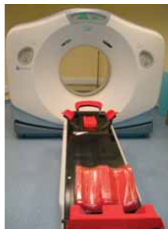
Wide-field-of-view CT scanner dedicated to treatment simulation
