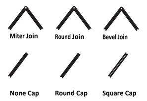
When using LINESTYLE2 for a miter join, a MiterLimitFactor must be specified and is used to calculate the maximum miter length:
