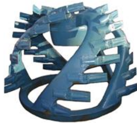
Figure 6. Pipeline dredge: midsize portable dredge (left) and cutter-head attachment (right).
