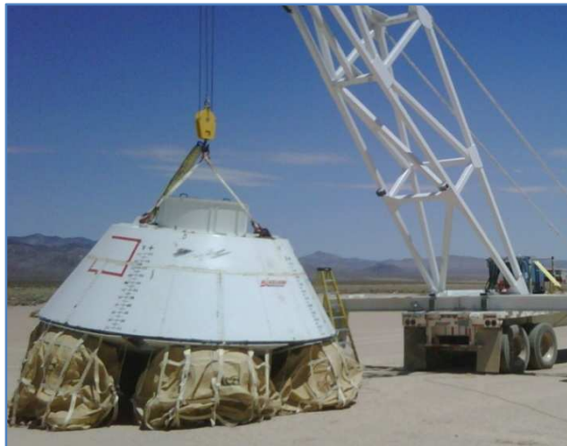
Figure 8. Mobile Air Bag Drop Platform. A mobile drop-test rig mounted on a flatbed truck, allows for the testing of the airbag landing system at planned landing sites with simulated wind velocities.
