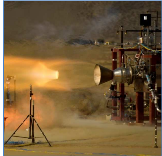
Figure 7 BANTAM Engine Testing. The BANTAM engine was tested in CCDev-1. In CCDev-2, an evolved configuration using bi-propellant fuels will be hot-fired.
