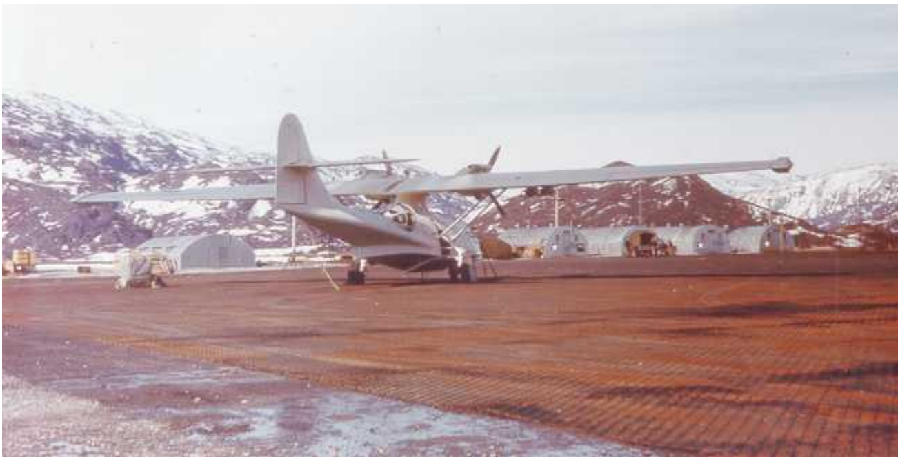
A Coast Guard PB5A of VP-6 at Bluie West 1, Greenland; note the Quonset huts in the background and the steel matting that served as the tarmac and runways on this isolated Arctic base.
