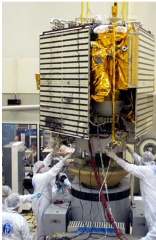
MESSENGER spacecraft during integration and testing. The sunshade is visible on the left with the spacecraft undergoing testing in thermal-vacuum conditions at NASA's Goddard Space Flight Center. On the right, the solar panels and Magnetometer boom are in their position for flight during work at APL.
