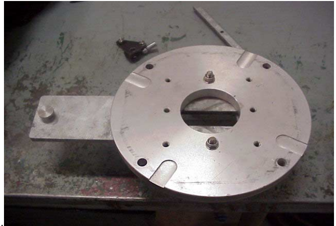
Fig. 3: Blocking device in blocked position
