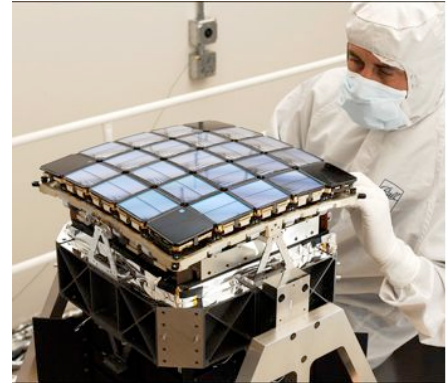
Figure J-2. The Kepler Focal Plane is curved with 42 1K x 1K CCDs.
