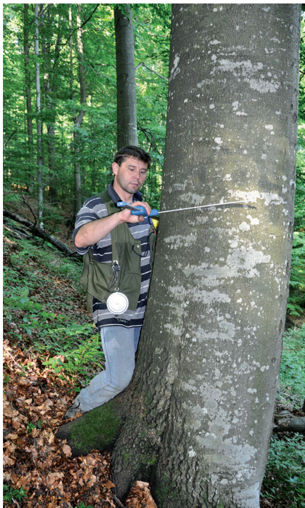
Fig. 3.1. Mykola Korol measuring the DBH of a large beech tree. The DBH was measured at a height of 1.3 m above ground. Photo R. Tinner.
