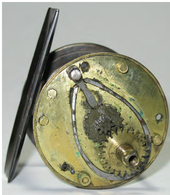
Charles Farlow's multiplying mechanism in tandem with a variable check c1860, which was the same as Ustonson fitted to the original model 100 years earlier.
