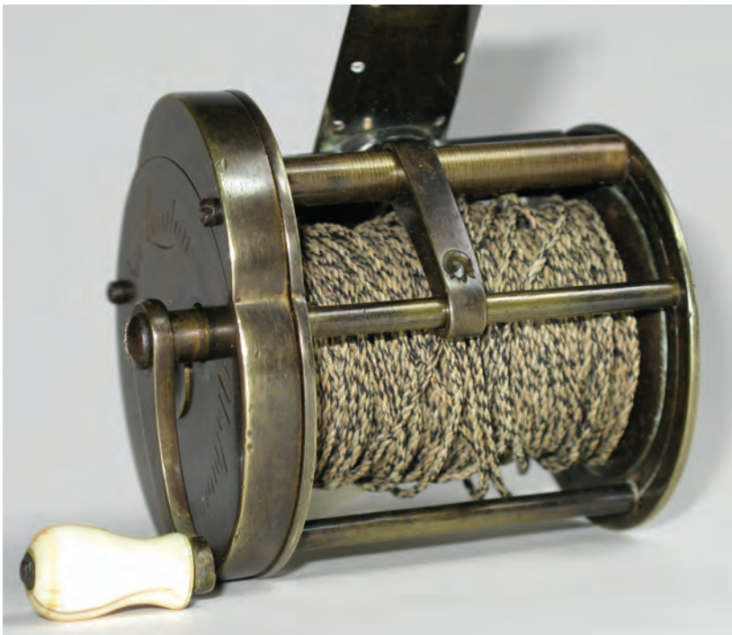
Line grooves in the soft brass rim of the guide made by the harsh abrasive horsehair line. Note the additional larger pillar along which the manual-level wind travelled.
