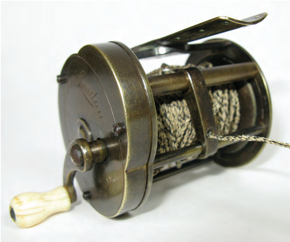
Ustonson's Original Multiplying Winch with the earliest line guide and manually operated level-wind. Set up with horsehair line, as it would have been used on the underside of a rod in the 18th century.
