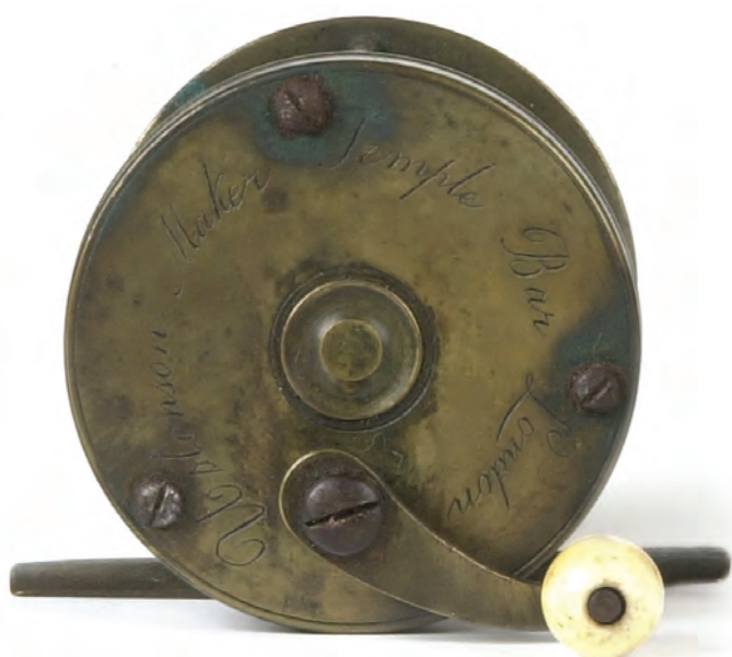
Ustonson multiplying brass winch 2¼" diameter, ivory handle on curved crank, faceplate engraved – 'Ustonson Maker, Temple Bar, London'. Multiplying mechanism in standard circular casing. (Angling Auctions)
