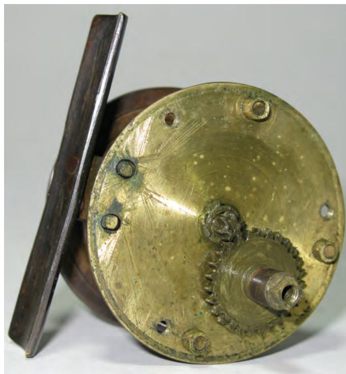
Early multiplying mechanism with the simpler two wheel gearing made by one of Ustonson's contemporaries.
