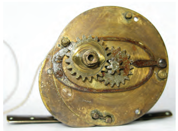
The first multiplying mechanism that worked in tandem with a reversible check to give a smooth and precise winding action, thus precision engineering as early as the 1760s. The multiplying mechanism has been fitted within the confines of a standard circular casing and the crescent shaped extension is empty.
