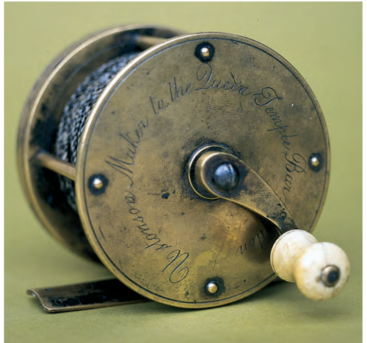
A brass winch of 2 \frac{3}{8} " diameter with curved crank and turned ivory handle, foot pierced with pad perforations. The handle plate with script engraving – ‘Ustonson Maker to the Queen, Temple Bar, London’.
