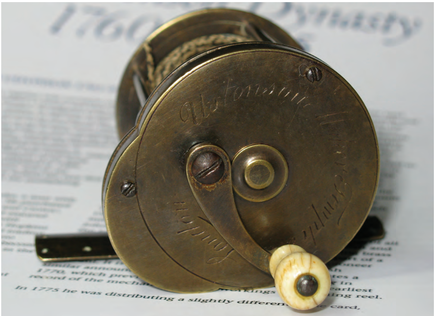
Ustonson's Original Multiplying Winch. It introduced the mechanism which marked the birth of bass fishing and bait casters of America, also generations of multipliers in Britain.
