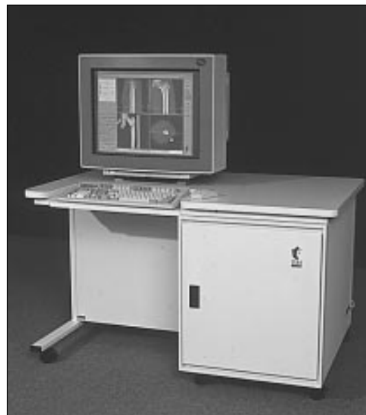
Plate 2 FDA-approved ORTHODOC, computer workstation, a pre-operative surgical planning system, develops a three-dimensional model of the bone
