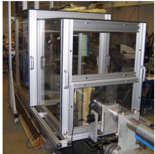
Figure 2. (a) PC Panel Mounting Setup for Impact Experiment and (b) Large Safety Enclosure
