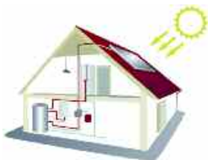
figure 9.3: flat panel solar technology
